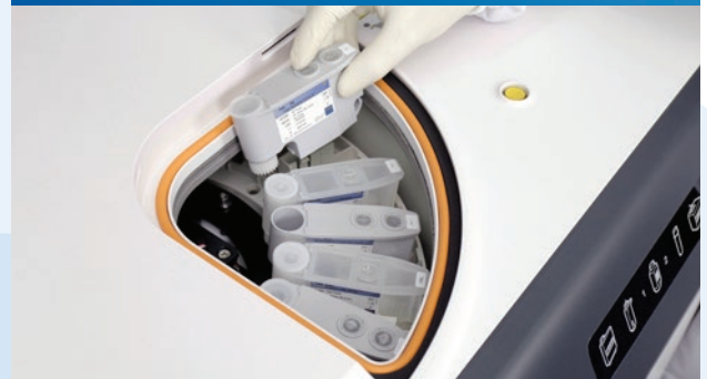
4. 25 reagent positions with 2-28°C refrigeration
