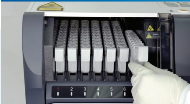
3. 70 sample positions with 1 min response time to STAT samples
