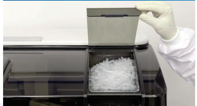
2. Bulk cuvette loading model with a maximum capacity of 1200 cuvettes
